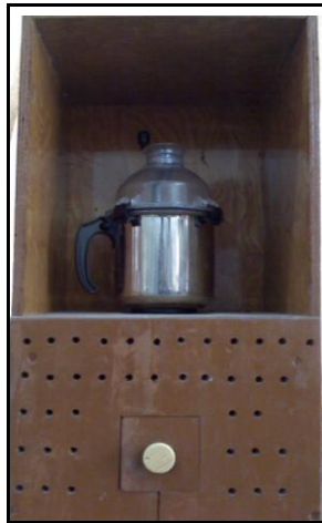
Fig 6. Photograph of Fabricated Slurry Erosion Test Setup.
